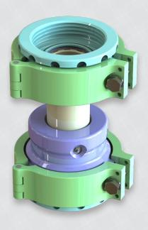
Premium's SDL-75 washpipe cartridge brings an economical hammerless solution to your top drive. The SDL-75 uses standard seals, but unlike conventional washpipes, the seals can be pre-compressed in the housing before installation.
