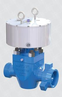
The Premium Oilfield Technologies AirForce™ mud gate valve provides the user with remote bleed-off capability of standpipe lines translating to a simplified and safer user interface. Utilizing the Premium NV-7500 core design allows our valve to be one of the longest lasting valves in the industry for applications up to 7500 psi.
